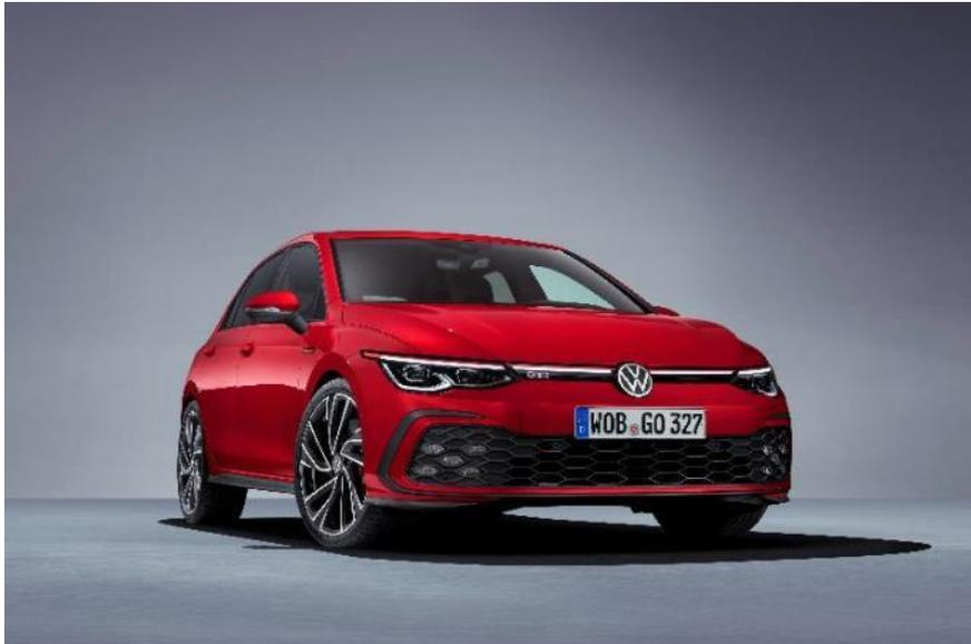
A classic with a new look: the Golf 8 with its new Volkswagen front light signature. Some models in the Golf 8 family are equipped with an LED strip across the front of the vehicle as standard. Its cover is made of impact-resistant PLEXIGLAS® Resist AG 100.
