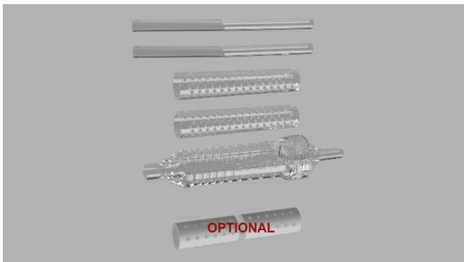
The patented BoneFlo®+ surgical handle consists of five injection-molded components made of CYROLITE®: a screw-on handle, which also serves as a filter housing, as well as two filters and two interchangeable suction tips. The synthetic bone substitute is available separately and can be used depending on requirements during an operation.
