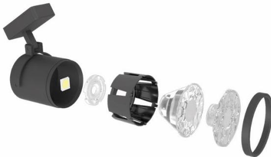
At the heart of the design (patent pending) is a special lens system comprising a collimator lens, which guides the LED light via total internal reflection (TIR), and a second, attached zoom lens.
