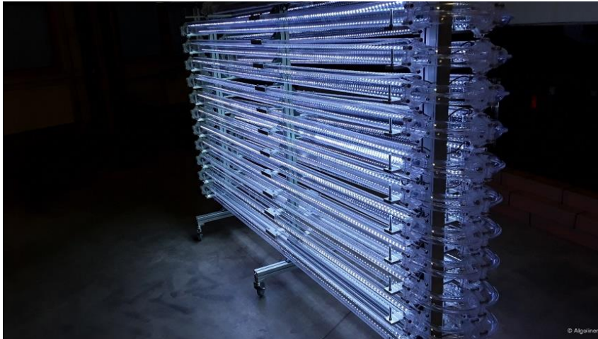
Algoliner test reactor made from ACRYLITE® tubes with integrated LED lighting. Photo: © Algoliner
